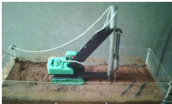
Figure 3. Piling Process Prototype Model
